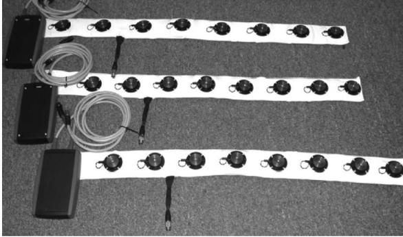
FIGURE 4 Three tactile display belt assemblies are shown along with their controller box.
