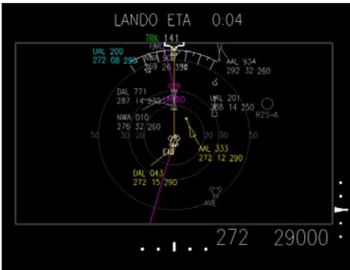
Figure 4. The Cockpit Display of Traffic Information (CDTI) used in the experiments supported by DATIDS. The illustration shows the ownership at the center of the display. The magenta line shows the own-ship's plotted path as derived
