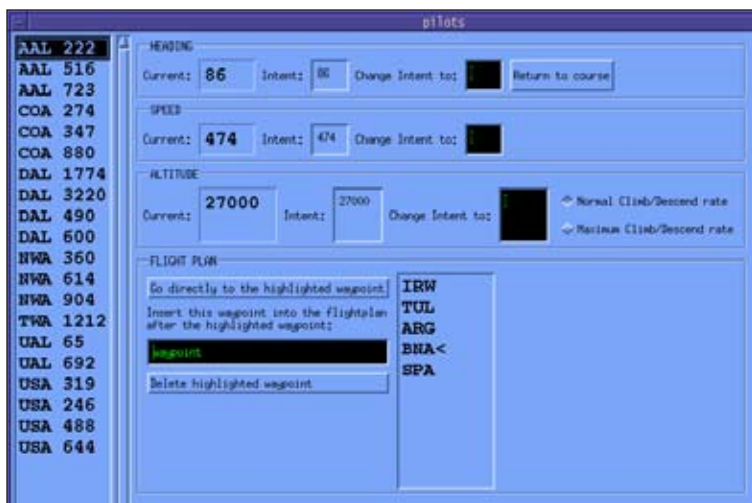
Figure 5. The 'Pseudo-Pilot' and Experimenter's Workstation enables real-time control of aircraft in the traffic scenarios. At left is a listing of all the aircraft in the scenario. Generally, only a subset of the aircraft on the list is present in the sec-
