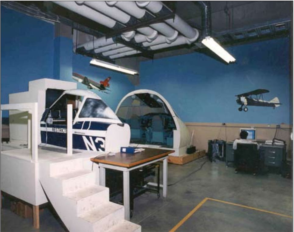
Figure 1. The Human Factors Research Laboratory's (HFRL, Univ. of Minnesota) Aviation Research Facilities. At the left, with the staircase, is a single-seat cockpit that housed a single (pilot) participant. Behind is a two-seat cockpit configuration. At right, one of the creators of the DATIDS system is seated at the ATC workstation.
