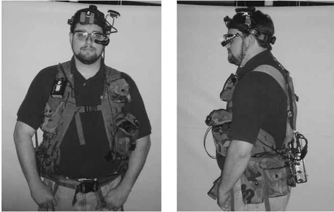
Fig. 1. Battlefield augmented reality system (BARS) used in the present study, front and side view.
