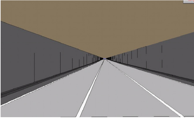
Fig. 3. A computer screen-shot of the no-pattern baseline experimental condition presented to participants. Note: thin vertical lines appearing on the tunnel walls are an anomaly of process by which this screen-shot was captured. Note: the image presented to participants in the driving environment simulator covered 165° field of view horizontally and 65° vertically.
