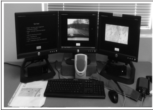
Figure 1. Experimental setup and simulation environment. Shown are three monitors, with a speaker mounted below each, and a keyboard with a mouse. Also displayed are the tactile belt with battery and a reference sheet describing visual targets that appear on screens two and three.
